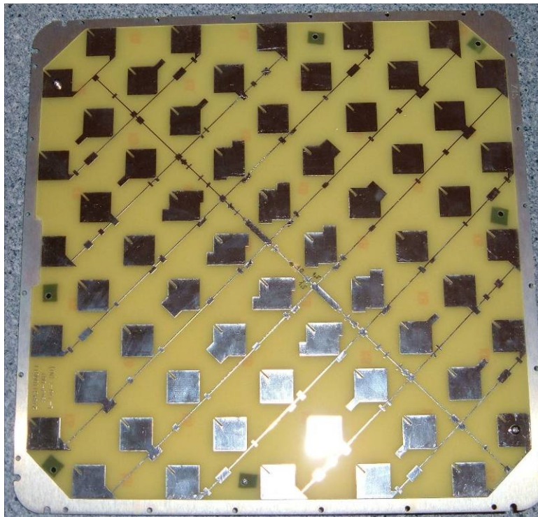
FIGURE 1.2: 5GHZ PANEL ANTENNA MADE OF AN ARRAY OF RADIATING PADS.
